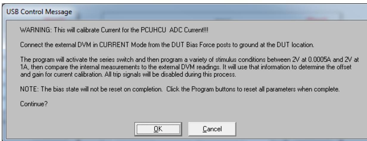
Figure 2-16: ADC Current Calibration Informational Box
