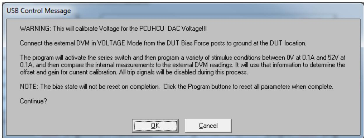
Figure 2-10: DAC Voltage Calibration Informational Box
