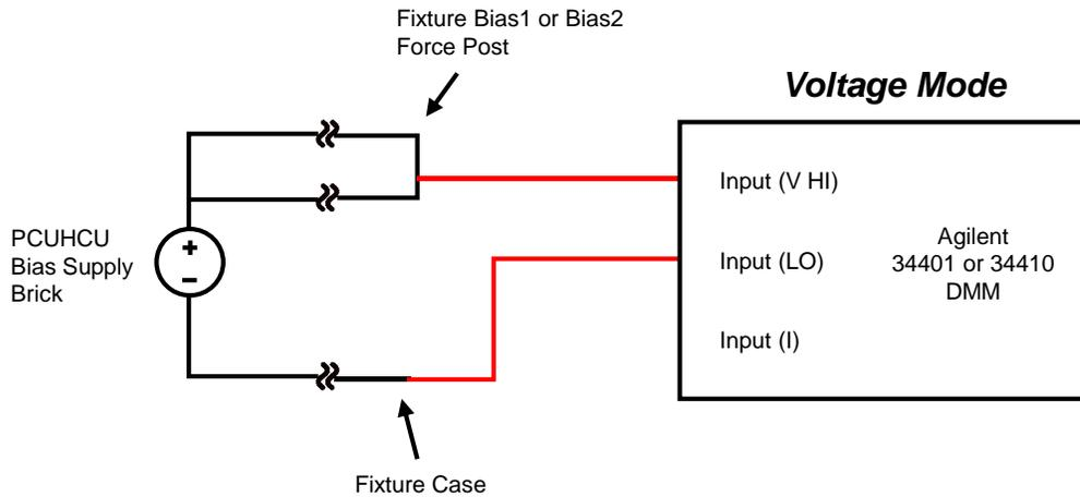
**Figure 2-7: Current Measurement Configuration**
